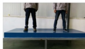
No deformation with 140KG
