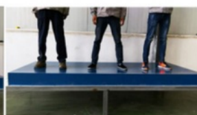
No deformation with 210KG
