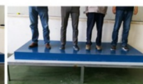
No deformation with 300KG
