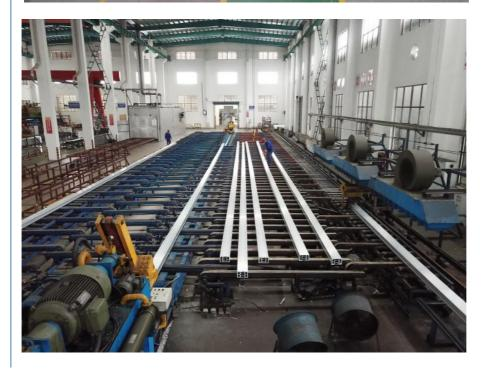
Tag: **LED Aluminum Heat Sink** extruded aluminum heat sink
